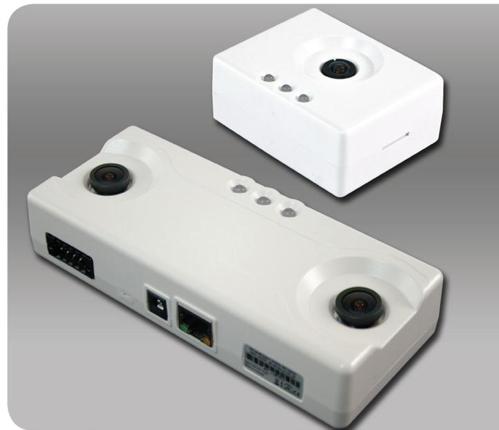
*BIC-1100 - Monocular Overhead Traffic Sensor*
